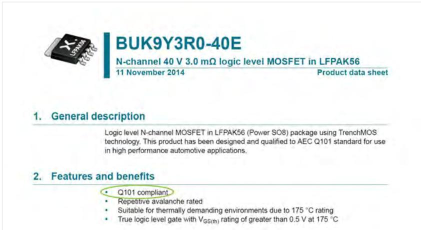
**Figure 5** | Front page of a typical Nexperia automotive data sheet, showing the MOSFET is automotive by highlighting that it is Q101 compliant
