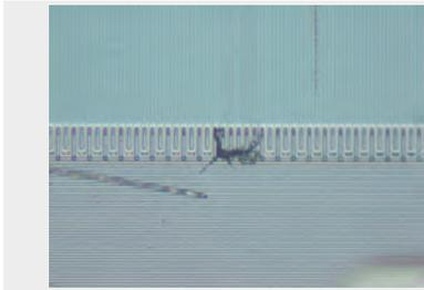
Figure 20 | Device 2 after Al, barrier and TEOS etch
