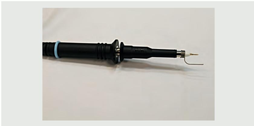
Figure 4 | Oscilloscope probe with ground spring attached
