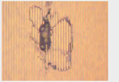
Figure 36 | Device 1 lower (orange) hotspot
