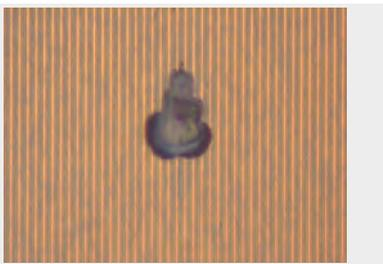
Figure 38 | Device 4 lower (orange) hotspot
