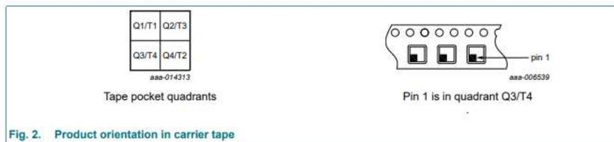
Fig. 2. Product orientation in carrier tape
